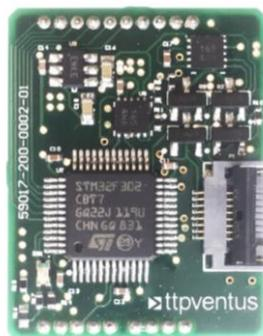
*Figure 2 – Disc Pump Drive PCB*
