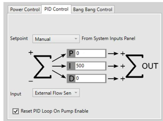
Figure 5: PID Control tab of the TTP Ventus Pump Control App
