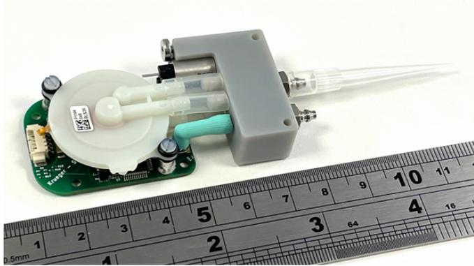
Above: prototype design for a Disc Pump pipetting module.
