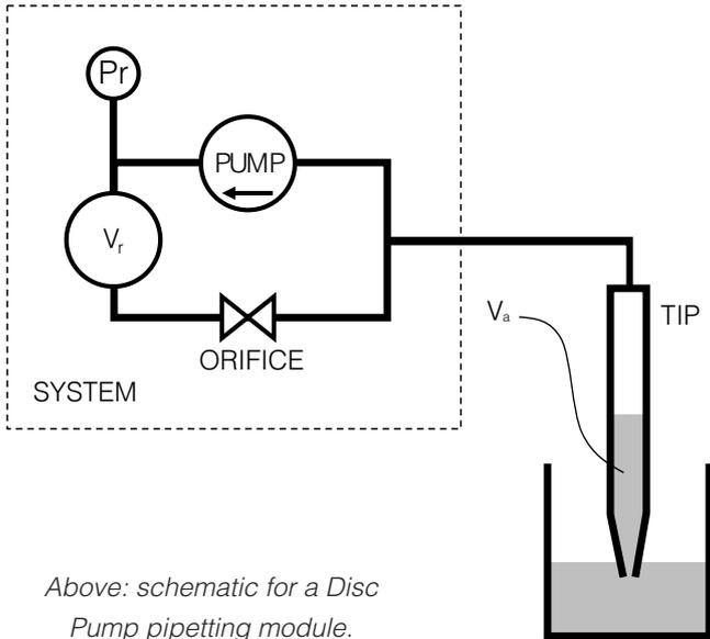
Above: schematic for a Disc Pump pipetting module.
