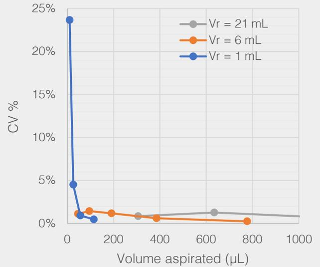
Above: repeatability data for aspirated volume for three reservoir volume sizes, demonstrating CV of ~1% or better over much of the measurement range.
