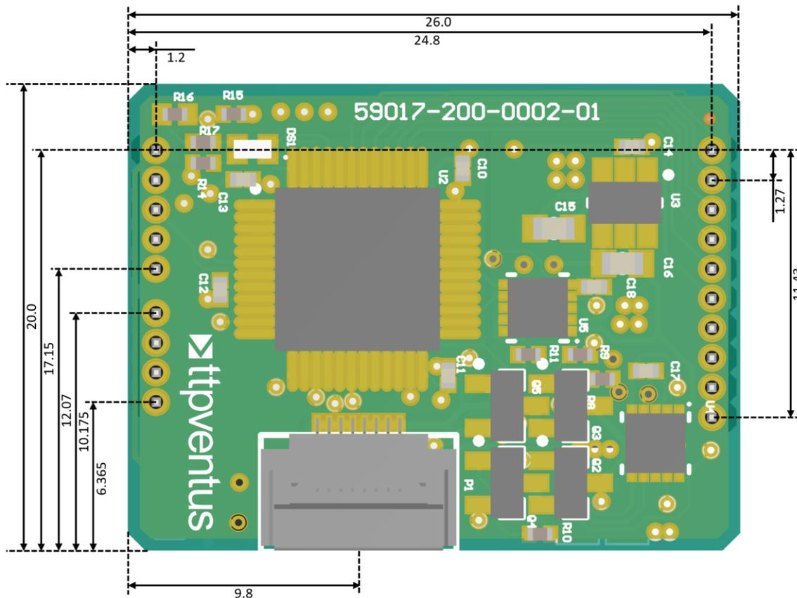
Figure 5 – Disc Pump Drive PCB dimensions (millimetres)
