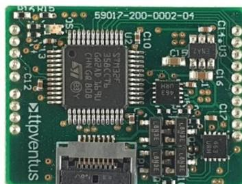
*Figure 2 – Disc Pump Drive PCB*
