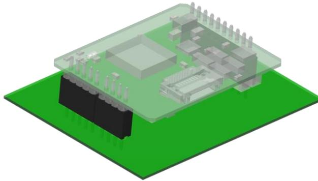
Figure 4 – Disc Pump Drive PCB mounted on a PCB
