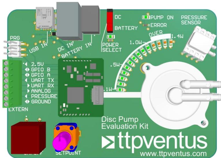
Figure 6 – TTP Ventus Disc Pump Evaluation Kit
